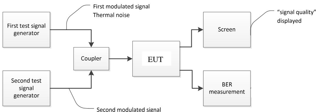
**Figure 10: Test arrangement - adjacent signal selectivity**
