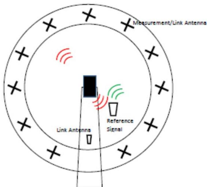
Figure B.7: Typical NFTF measurement setup
