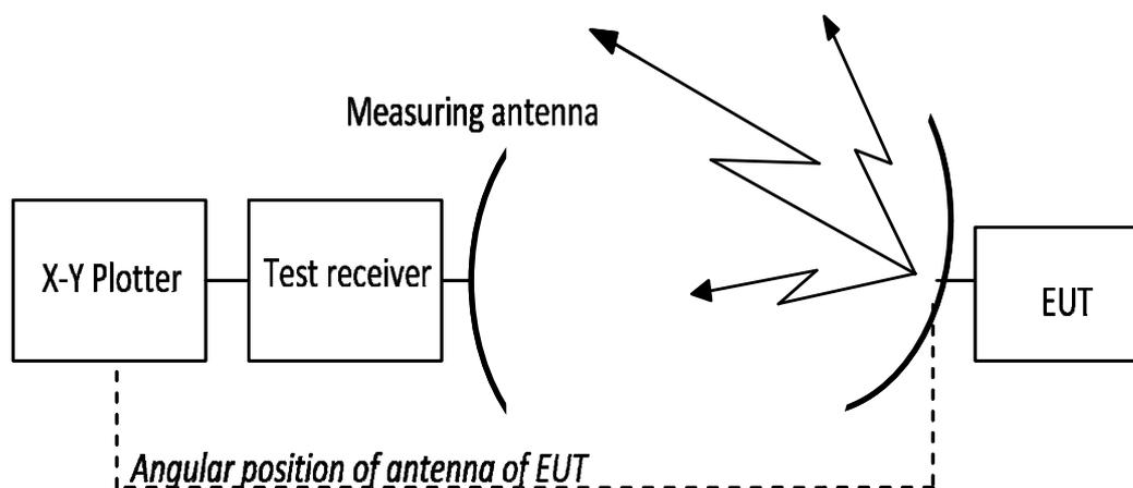
**Figure 8: Test arrangement - antenna beam pointing**
